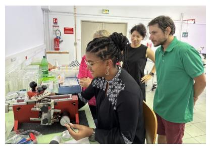
Training on section preparation using sliding microtome
